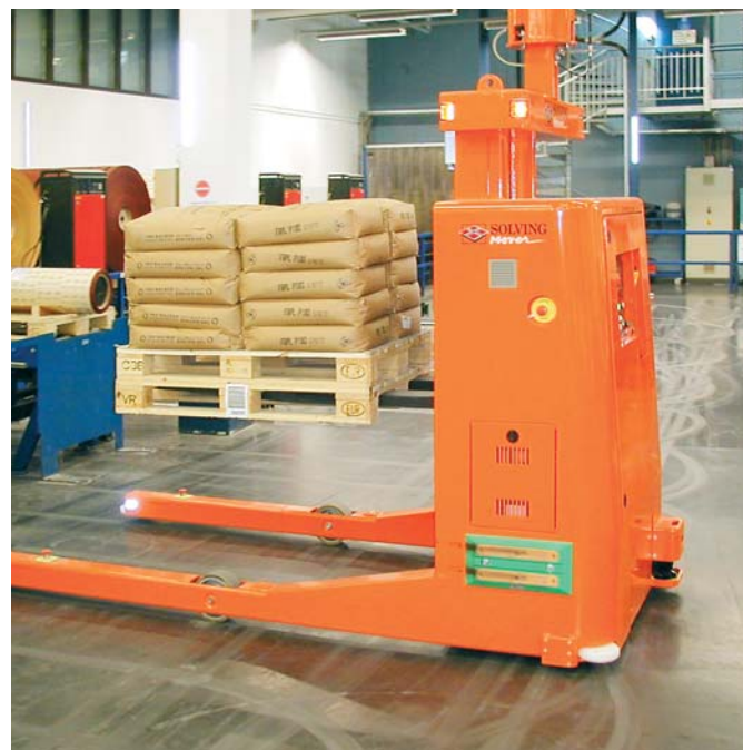
The Solving AGV Pallet Mover has a capacity of 2 000 kg.
