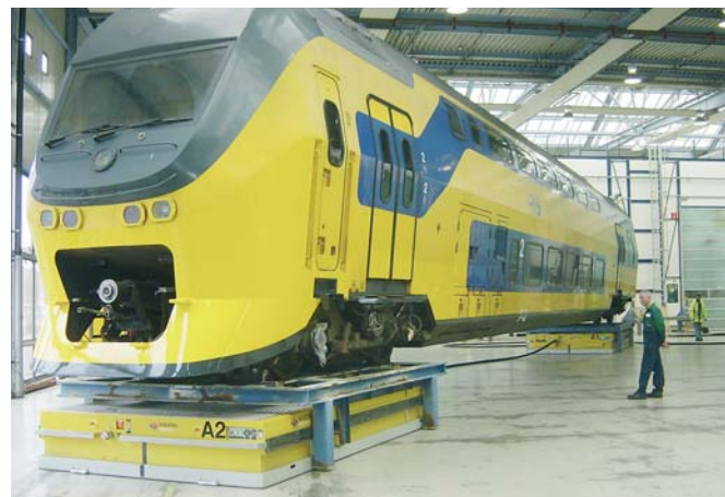
Solving air film-based Movers are used during repair and maintenance.
