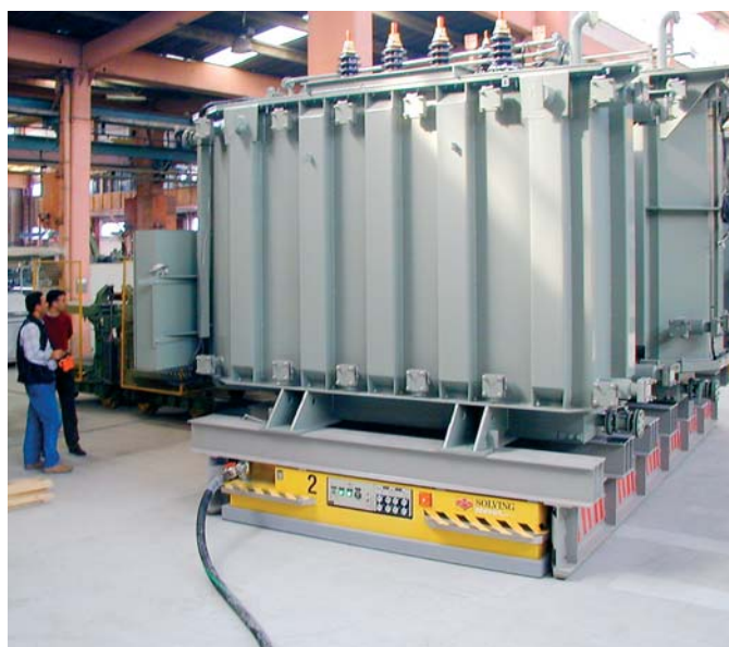
BEST A.S. in Turkey has installed a Solving air film Mover to move large transformers quickly and smoothly through production and test facilities.
