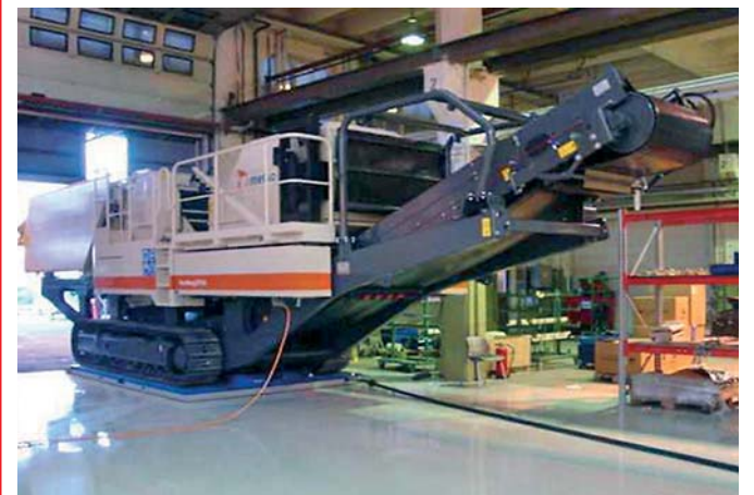
Mobile crushers are floated on air bearings through an assembly line consisting of five stations.
