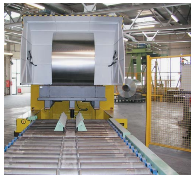
The Solving AGV Mover assisted Hydro Aluminium in finding a practical solution to their requirement for regular material flow between buildings.
